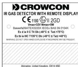
IRmax with IS Barrier certification label
