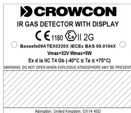
IRmax with Fixed IR Display certification label
